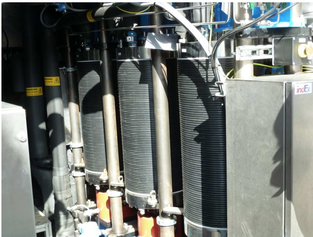
Figure 6.3: Electrolyzer stacks to produce Hydrogen for grid injection from renewable power in a pilot plant in Frankfurt
