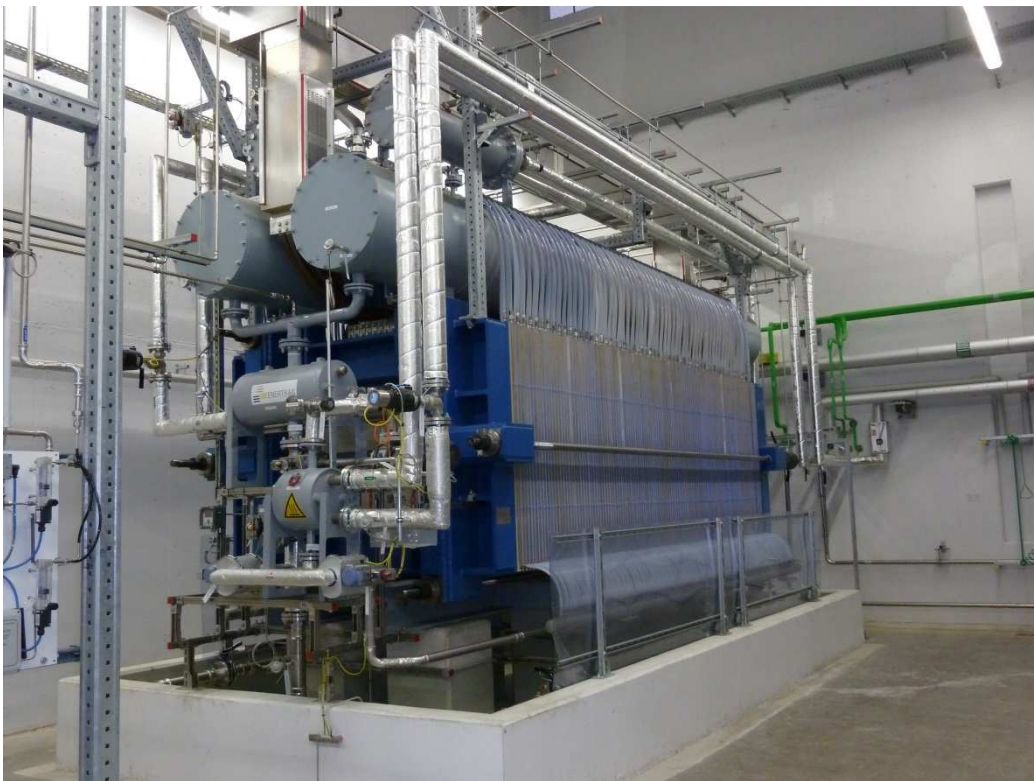
Figure 6.4: Large scale electrolyzer producing hydrogen for methanation
